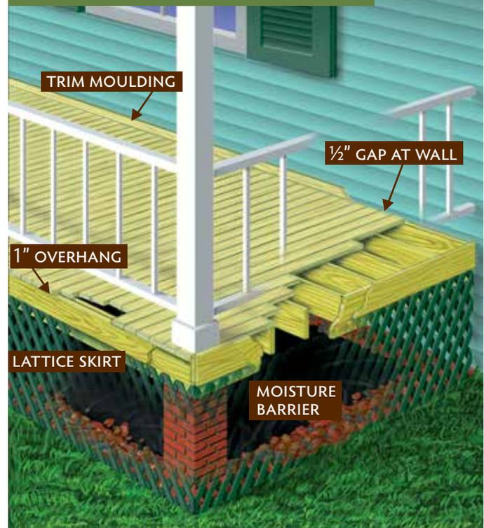
Attention to proper porch design is as important to the longevity of the structure as are the details of porch flooring specification and installation. Inadequate air circulation beneath the porch and trapped moisture between framing components will greatly reduce the serviceability and long-term appearance of the porch. The following recommendations are key elements to the proper design and construction of a fully-covered porch:
